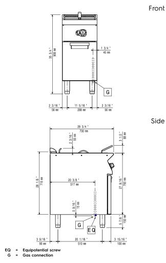
GasGas Power:14 kWStandard gas delivery:G30 - 50 mbarGas Type Option:G31 37 mbarGas Inlet:1/2"
